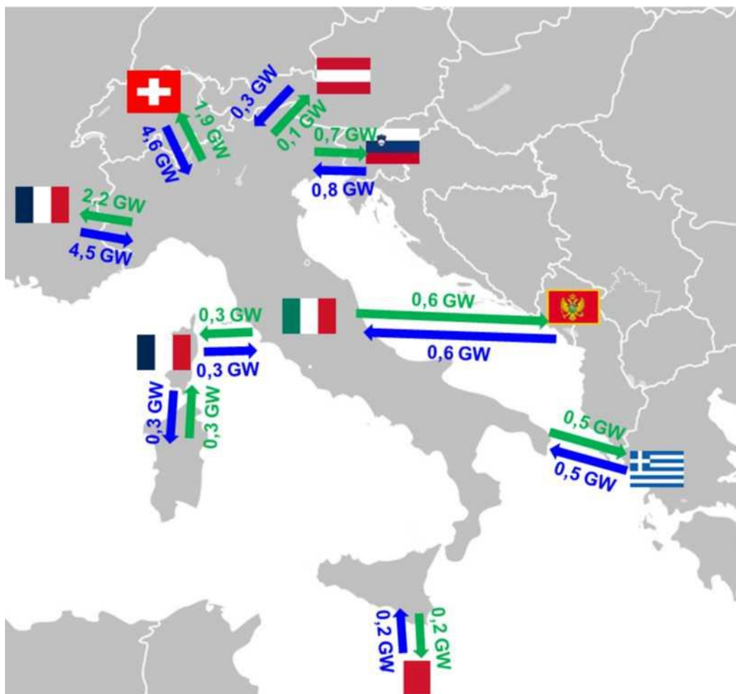
Figure 1 – Cross-border import and export trading capacity of existing interconnections (maximum NTC 2023 processing and transit limits – source Terna)
