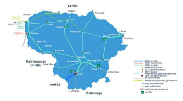
Figure 4.5.2.2. 400-330 kV transmission network in 2031, when Lithuania's EES will work synchronously with KET<sup>114</sup>
