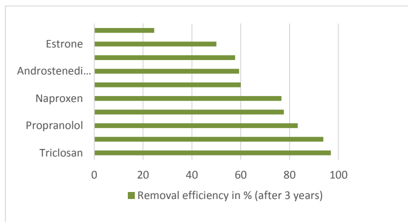
Figure 19: Removal efficiency rates after 3 years of a constructed wetland (Source: Vystavna et al. )
