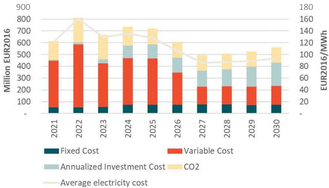
Figure 5.7. Average cost of electricity and breakdown of system cost elements – AFM.
