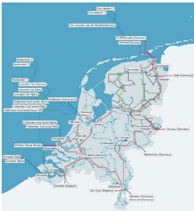
Figure 4.11 Transmission Network and Interconnectors (Source: TenneT,
