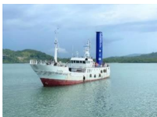
Figure 5: Aspiring wingsails - Balueiro Segundo vessel
