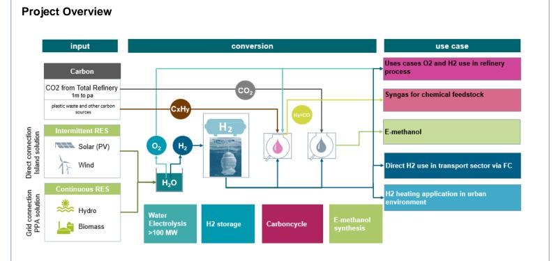
Siemens Technology: Silyzer 300, H2 compression) Main Partners: Linde, Fraunhofer
