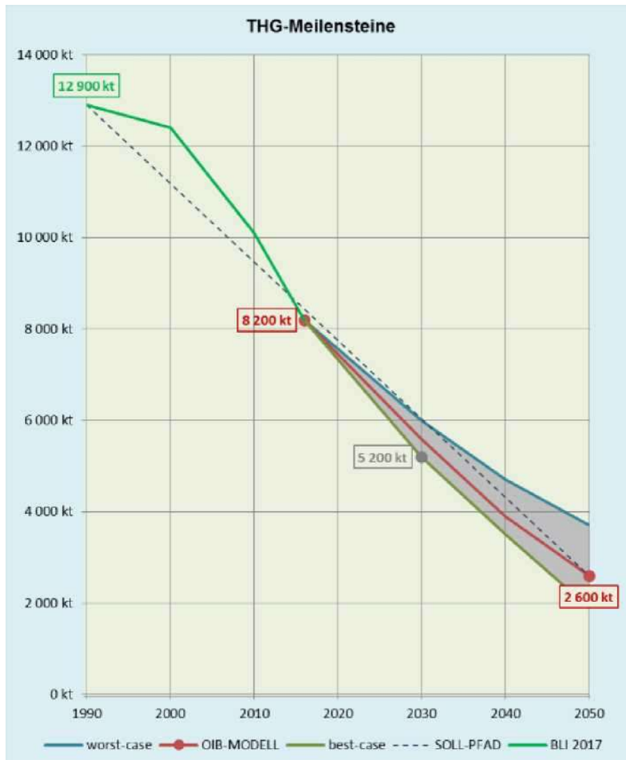
Figure 16: GHG milestones (in 1 000 tonnes = kt CO 2 equivalent) in accordance with OIB LTRS April 2020; Changes for coal, heating oil, district heating, heat pump, electricity, biomass and solar heat and natural gas as a residual value for the development of the energy mix expected by the Länder
