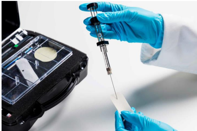
Figure 1.4-1. JRC has developed a test kit to verify the performance of Explosive Trace Detection (ETD) equipment at the airports. The test kit is now used across European airports and has become a de facto standard for the performance assessment of ETD equipment.
