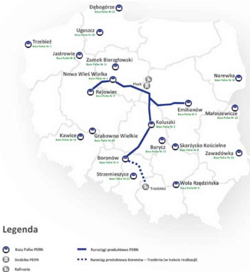
Figure 2.29. Illustrative layout of PERN S.A. product pipelines (as of 2023)
