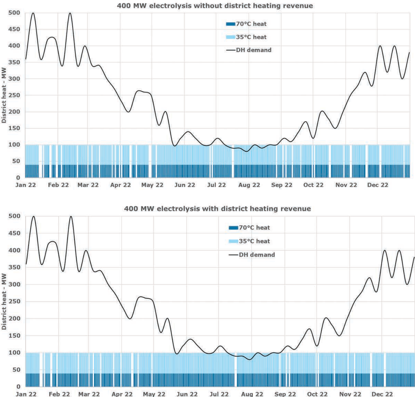
Figure 7. District heating production in a large system with waste heat from electrolysis. Top: operating profile without revenue from district heating. Bottom: operating profile with revenue from district heating. The additional operating hours due to district heating are evident from the smaller number of white gaps in the bottom profile.
