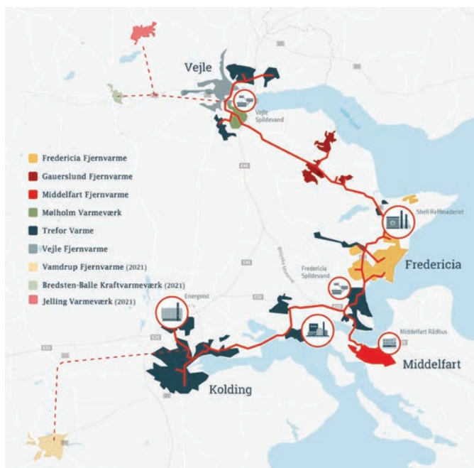
Figure 19. Heat transmission in the Triangle Region combines heat production and local district heating areas via the TVIS district heating transmission grid (red lines). Source: TVIS.net
