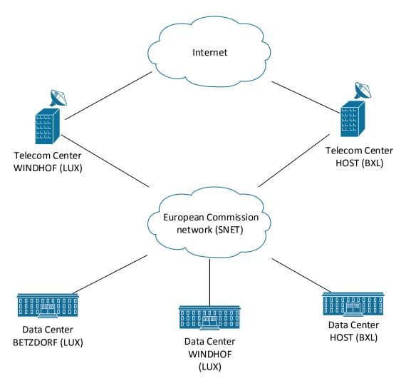
The telecom centres (TC) do connect the European Commission Network (SNET) to a number of different networks, including the Internet. The exact nature of all these connections is irrelevant for the purpose of the present tender, except for the SWIFT connectivity, which is the object of this tender.
