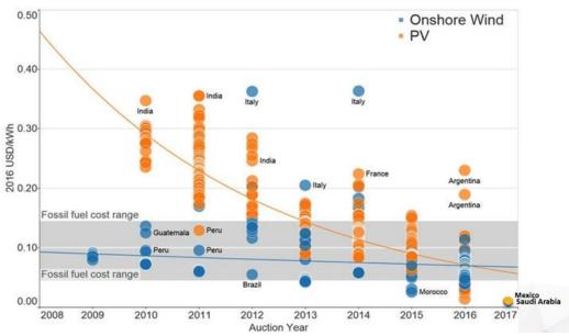
The cost reduction progress for PV results in ever lower LCOE\*
