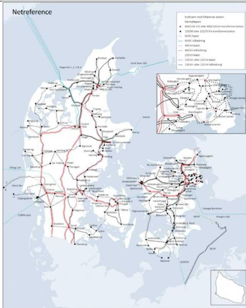
Figure 56 Net Reference for 2030, including existing electricity grids and approved maintenance or extension projects
