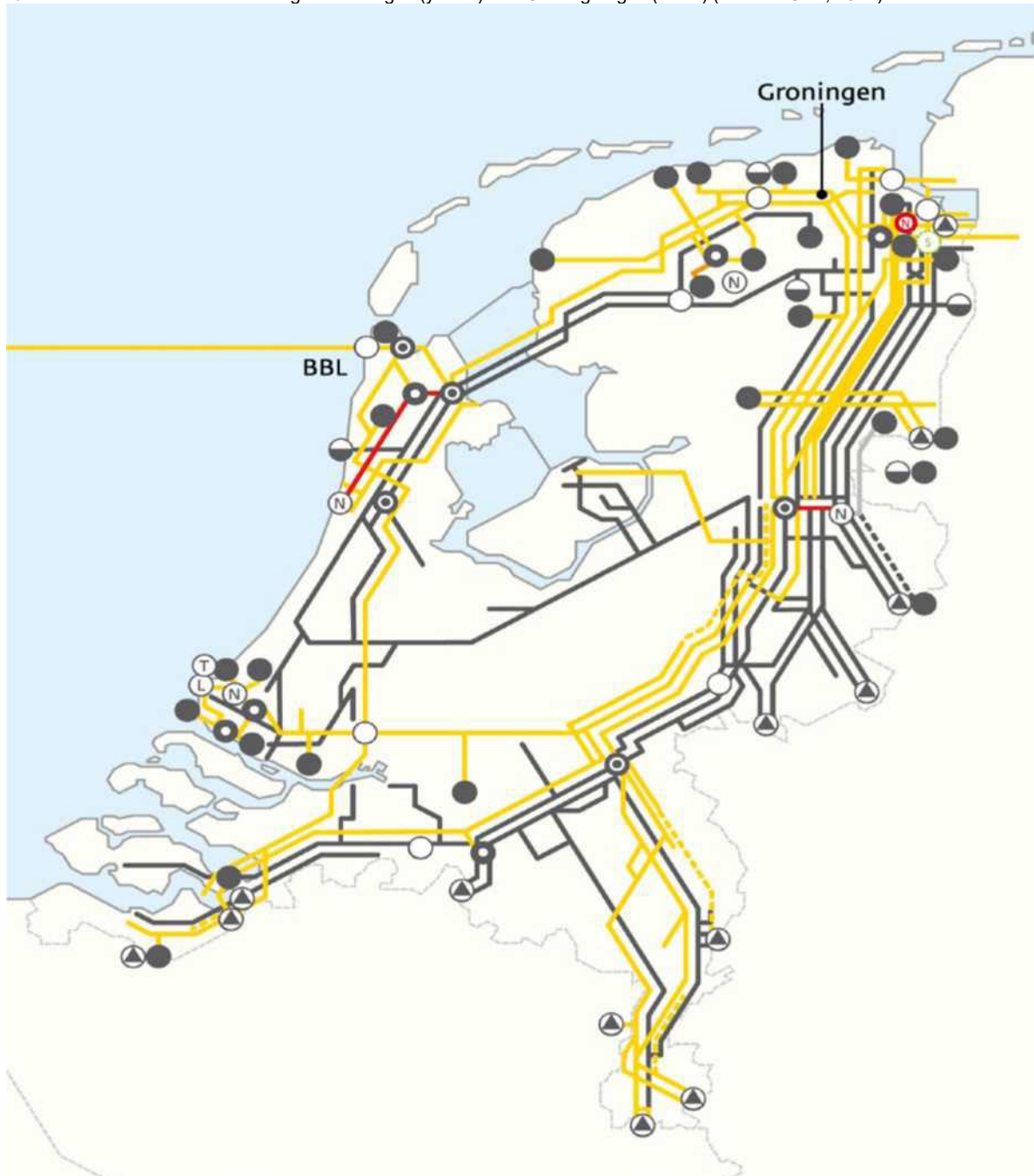
Figure 4.12 transmission network for high calorific gas (yellow) and Groningen gas (black) (Source: CTS, 2022)
